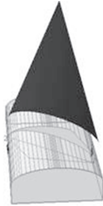
Fig. 2-2. Exposed area of a block in the roof
